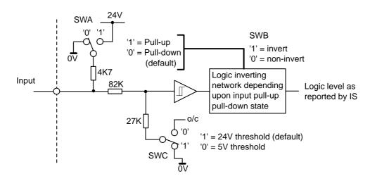
Figure 3-14. User Input Circuit
